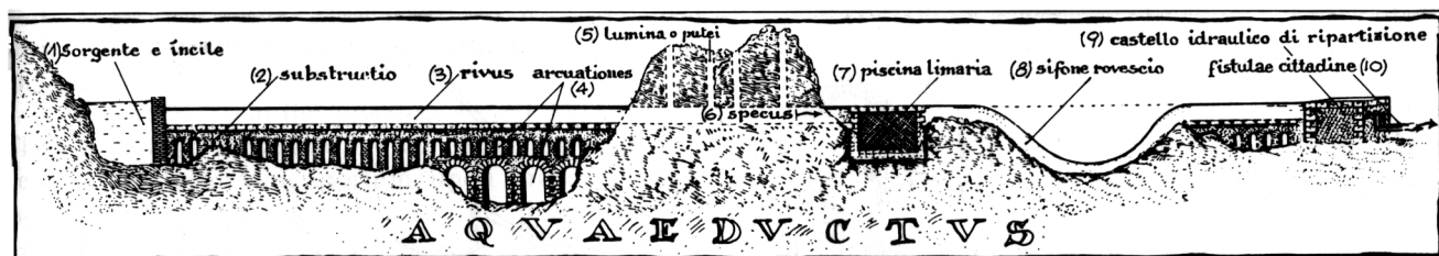
Fig. 1 Section of a Roman aqueduct: (1) spring and inlet; (2) bearing wall; (3) open channel; (4) arcades; (5) shafts; (6) underground channel; (7) settling basin; (8) reverse siphon; (9) main reservoir; (10) water pipes
